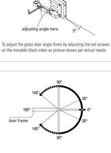
Door closing speed adjustment from  $30^{\circ} - 0^{\circ}$ , loosen No.2 valve counter-clockwise to speed up, tighten No.2 valve clockwise to slow down. 1 mm higher than the hole is prohibited while adjusting No.2 valve.
