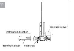
Open the door at 90°, mount the base back cover vertically at the end and the base front cover horizontally at the front. Align the side holes of base front cover with the screw holes on base side, screw out the set screws by Allen key to fix the base cover.
